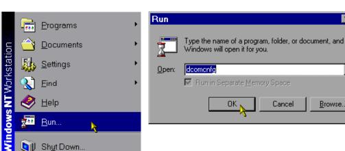
DCOM Config (known DCOMCNFG.EXE) is a utility that can be used to secure Distributed COM (DCOM) objects that have been created.
