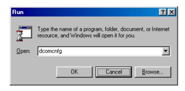
DCOM Config (known as DCOMCNFG.EXE) is a utility that can be used to secure Distributed COM (DCOM) objects that have been created.
